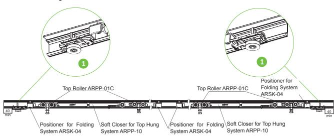
2 Insert the doors into the tracks and adjust them. Insert the cable and fix it by turning the hexagon bolts. Adjust the Soft Closers, the Positioners and install the Top Track Cover CKRU0592.
